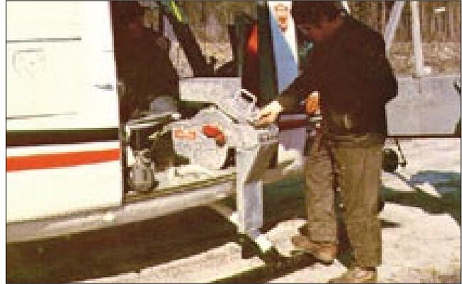
Delayed Aerial Ignition Device (DAID) mounted in a helicopter. Photo: Bugwood.org.
