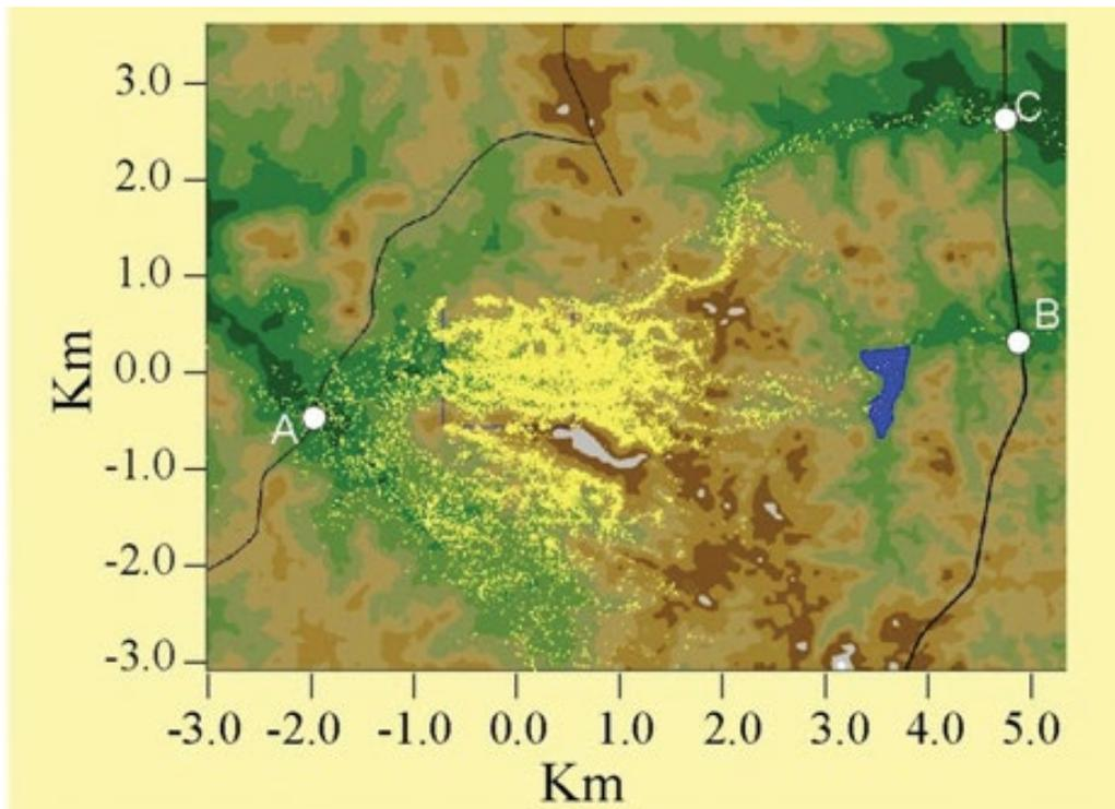
Sample output from PB-Piedmont showing smoke (yellow particles) moving down drainages and crossing roads at points A, B, and C.
